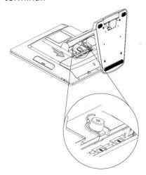
3) Loosen the butterfly screw from the back of the stand and remove the dummy cover.
