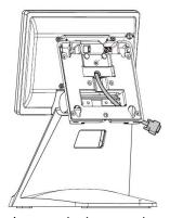
5) Attach the stand to the terminal and secure it with the thumbscrew. Connect the VGA cable to the VGA port on the terminal.
