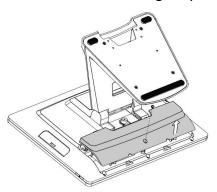
2) Loosen the thumbscrew and slide the stand towards the I/O ports to release from the terminal.
